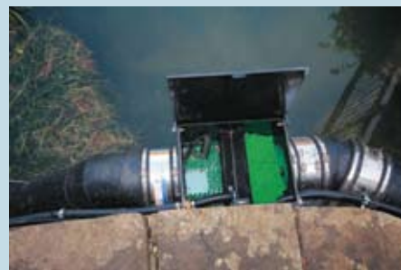
The header box with lockable lid in the open position. The camera is visible in the middle of the left hand section at the top
